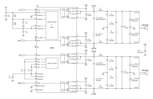
NOTE 1:  $C_{SN}/R_{SN}$  are optional locations, loaded only if required to reduce overshoot
