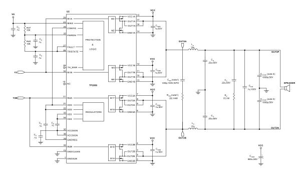
NOTE 1:  $C_{SN}/R_{SN}$  are optional locations, loaded only if required to reduce overshoot
